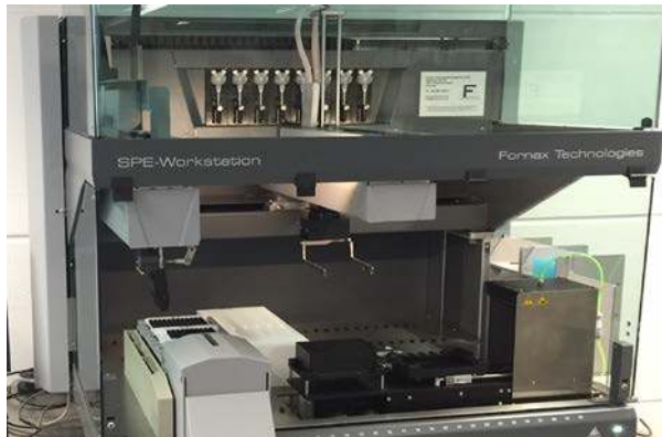
Base: Tecan EVO® 100 with Fornax SPE Processor , LiHA and RoMa
